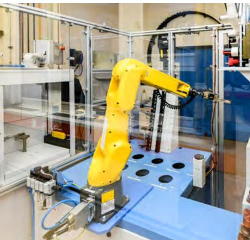
**This robot analyzes stamping samples fully automatically.**
